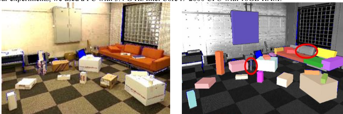
Fig. 11. Reconstruction of box shapes. (a) points with colors, and (b) extracted box shapes.
