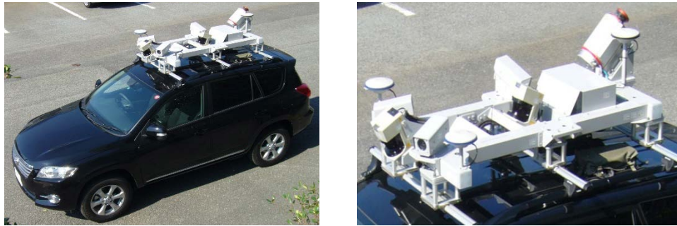
Fig. 1. Mobile Mapping Systems. (a) Vehicle with an MMS, and (b) Close-up of MMS.
