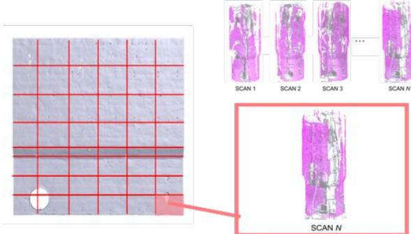
Fig.16: Cells generated by dividing the wall surface
