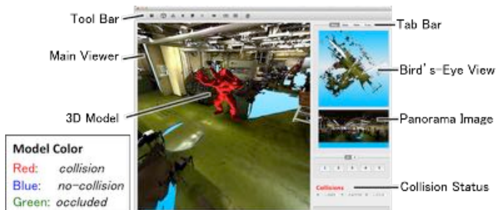
Fig. 4: Collision detection system
