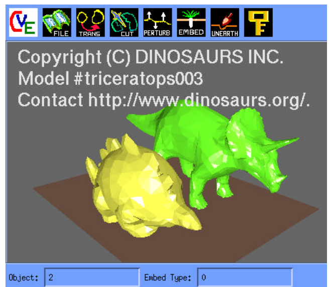
Figure 1. Three-dimensional models of dinosaurs in this scene are embedded with copyright notices and contact addresses, which can be extracted and displayed on demand.
