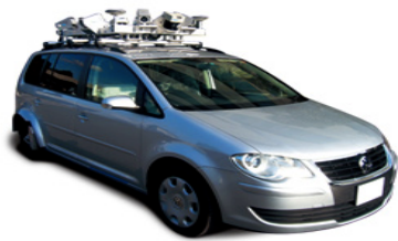
Fig.1 Mobile Mapping System
